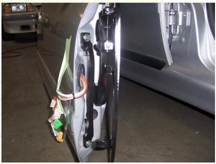
to make the wires go in a straighter layout towards the front of the door. After gaining the desired wire slack use zip ties to secure the wires to the door.
