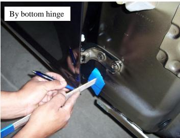
Once you have found the factory location of your door you now can remove the door so that you can install the new VDI hinge as shown on the right.
