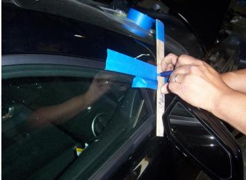
You will also need to measure and mark the distance of the edge of the door to the body as shown below.
