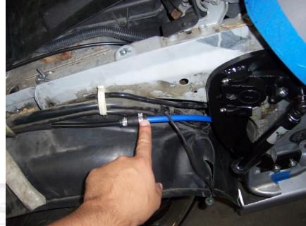
The emissions canister will have to be reposition under the radiator reservoir tank.
